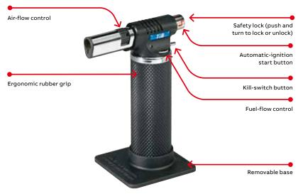
Portable heat shrink torch Separate fuel- and air-flow controls enable precise adjustment of flame and temperature to 1,371 °C (2,500 °F).
